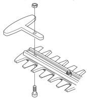
Use the screw and the nut on the cutting deck. Tighten to 8 Nm.
